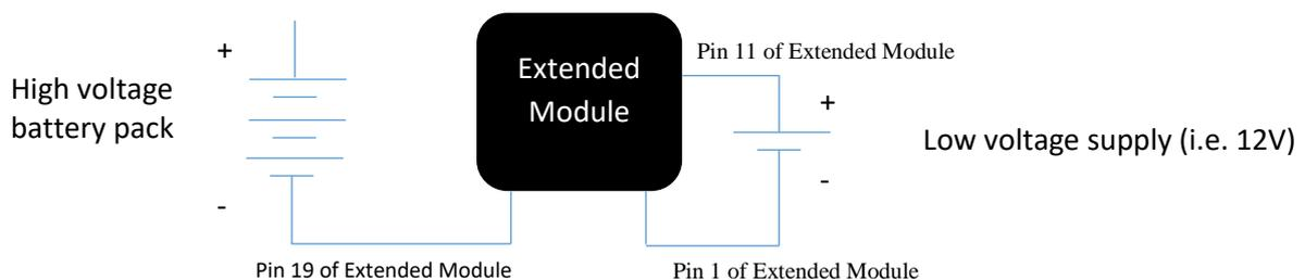
Figure 4 – Isolation resistance connection circuit
